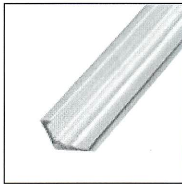
Model FLG H •H-rated Flange •22-gauge galvanized steel •Meets SMACNA rigidity Class H for transverse joints (steel)
