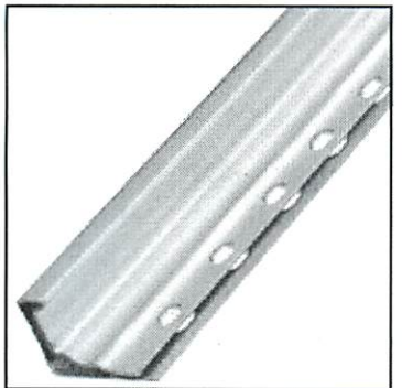
Model Q FLG J QUICK FLANGE™ •J-rated Flange •20-gauge galvanized steel •Meets SMACNA rigidity Class J for transverse joints (steel) •Meets SMACNA rigidity Class H for transverse joints (aluminum)
