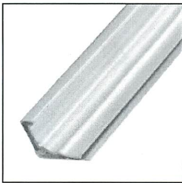
Model FLG J •J-rated Flange •20-gauge galvanized steel •Meets SMACNA rigidity Class J for transverse joints (steel) •Meets SMACNA rigidity Class H for transverse joints (aluminum)
